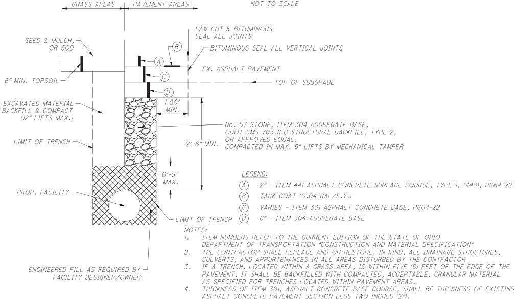
5. ASPHALT BIKE PATH PAVEMENT SECTIONS SHALL CONSIST OF LEGEND ITEMS (A) & (D)
