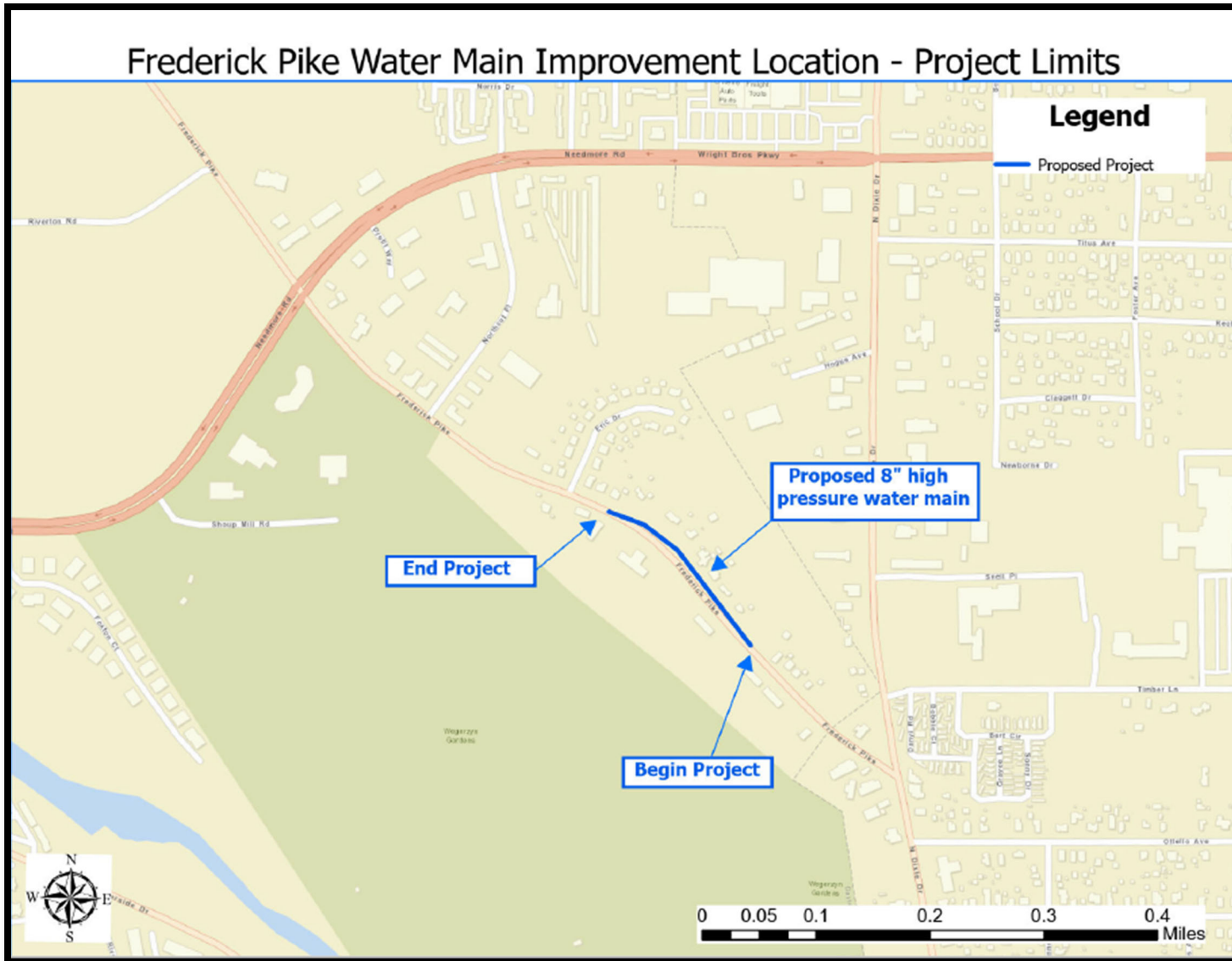
Figure 2-Frederick Pike Water Main Improvements Project Limits
